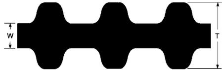
**Fig. 37 Twin Power Belt Tolerances**
